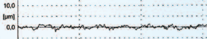
Surface roughness profile Ra approx. 0,5 µm
